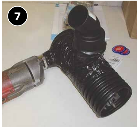
7 Utilize hand tools and/or shrouded tools attached to a HEPA vacuum that minimize dispersion of dust and debris.
