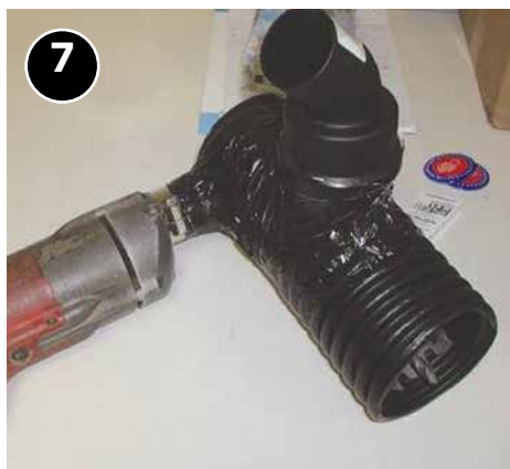
Use hand tools or shrouded power tools attached to a HEPA vacuum to limit the spread of dust and debris.
