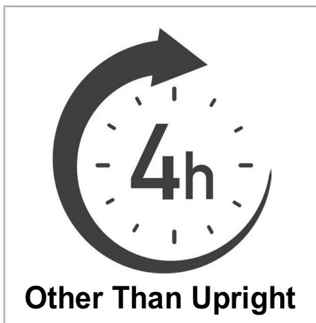
If the refrigerator was transported upright, wait 1 hour before plugging it in and turning it on. If the refrigerator was transported in an orientation other than upright, most manufacturers will recommend you let the oil in the compressor settle in its upright position for 4 hours before plugging it in and turning the unit on.
