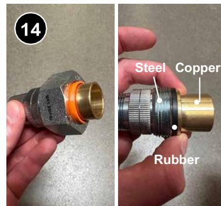
Install dielectric unions when connecting copper to galvanized steel piping in accordance with IRC and manufacturer specifications. [7.0302.6i.](#)
