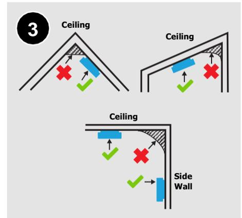
Avoid installing in locations with dead air space, or locations with excessive fresh air inlet (i.e., frequently used doors and windows).
