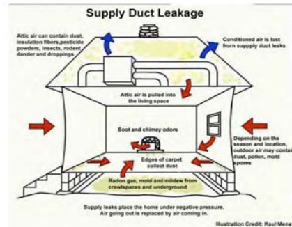
This illustration depicts the potential consequences of leaks on the supply side of the duct system. The volume of air that leaks out into the attic creates negative pressure imbalance in the home causing the problems shown.
